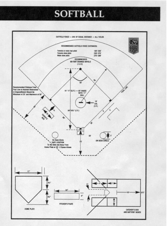
When laying out the softball diamond, it is recommended that the line from home plate through the pitcher's plate to second base run east-northeast.
